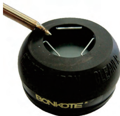
Simple residues can be cleaned off the tip at the rubber lip
